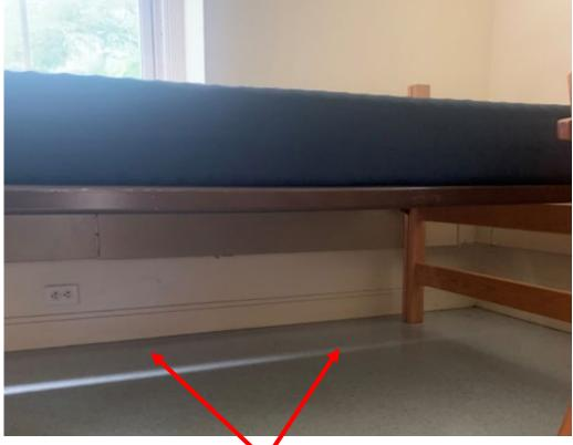
The area below this bed is clear and allows the proper flow of air through the heater. Please do not clutter the area below the bed with boxes or storage bins which can block the airflow.
